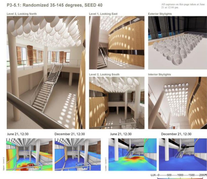
Figure 10: Design interventions explored with Grasshopper software include variable cowl depth (2' to 4'), and orientation (45 or 65 degrees north or south of east), Renderings by Julie Oelkers.
